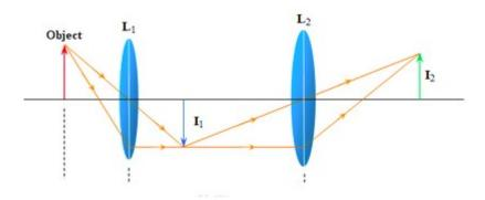
The image of the first lens  $I_1$  becomes the object for the second lens  $O_2$
