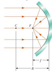
The mirror equation enables one to calculate the image position from the object position and the radius of curvature of the mirror.
