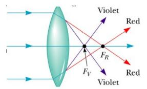
There are technical ways of reducing chromatic aberration, including the use of compound lenses consisting of converging and diverging lenses.
