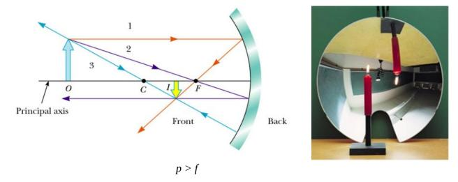
As can be seen from the diagram, the image is inverted and reduced in size.
