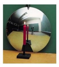
By extrapolation to the back side of the mirror, the reflected rays intersect to define the image on the back side. The image is upright and reduced in size. It is virtual since the reflected rays do not actually pass through the image.
