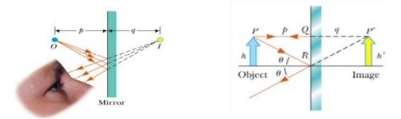
The object distance is *p* and the image distance is *q*. For flat mirror, p = q
