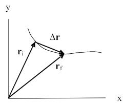
The velocity is always in a direction tangent to the path.
